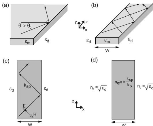
Fig. 1. Dielectric waveguide treatment of surface polaritons along finite interfaces: (a) TIR of a surface polariton wave, (b) ray-optics interpretation of a surface polariton mode, (c) top view of the ray-optics interpretation, (d) equivalent two-dimensional dielectric slab waveguide.
