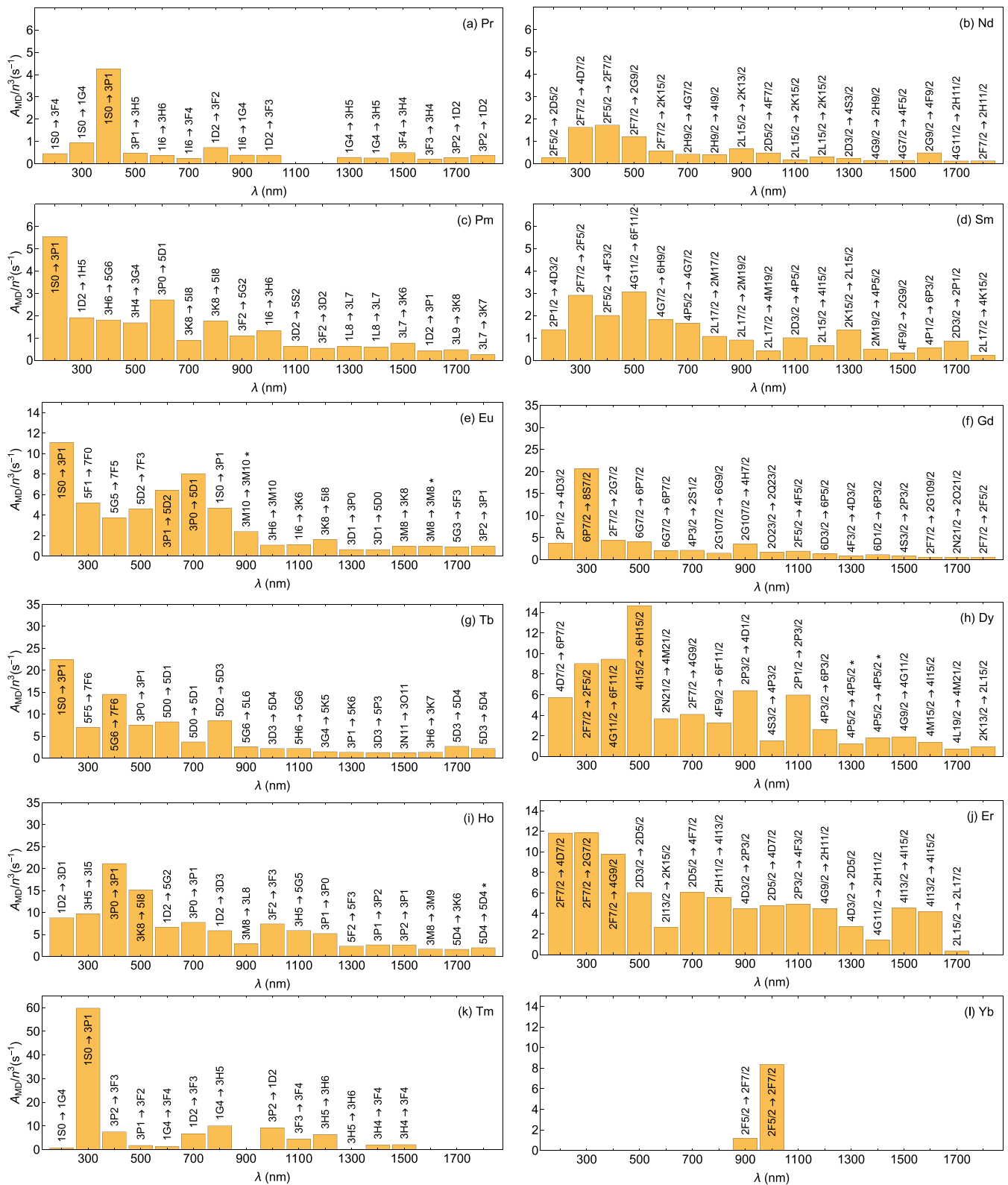
FIG. 8. Maximum magnetic dipole transition rates for different wavelength ranges across the lanthanide ions. The height of the bar indicates the magnitude of the rate and the text shows the main (2S + 1)LJ component of the initial and final states. Cases marked with * are cases in which the given coarse labels are ambiguous, see Table IV for a longer description of these cases.
